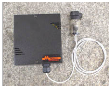
Pressure Relief Valve Monitoring (Tee'd off vent pipe)
