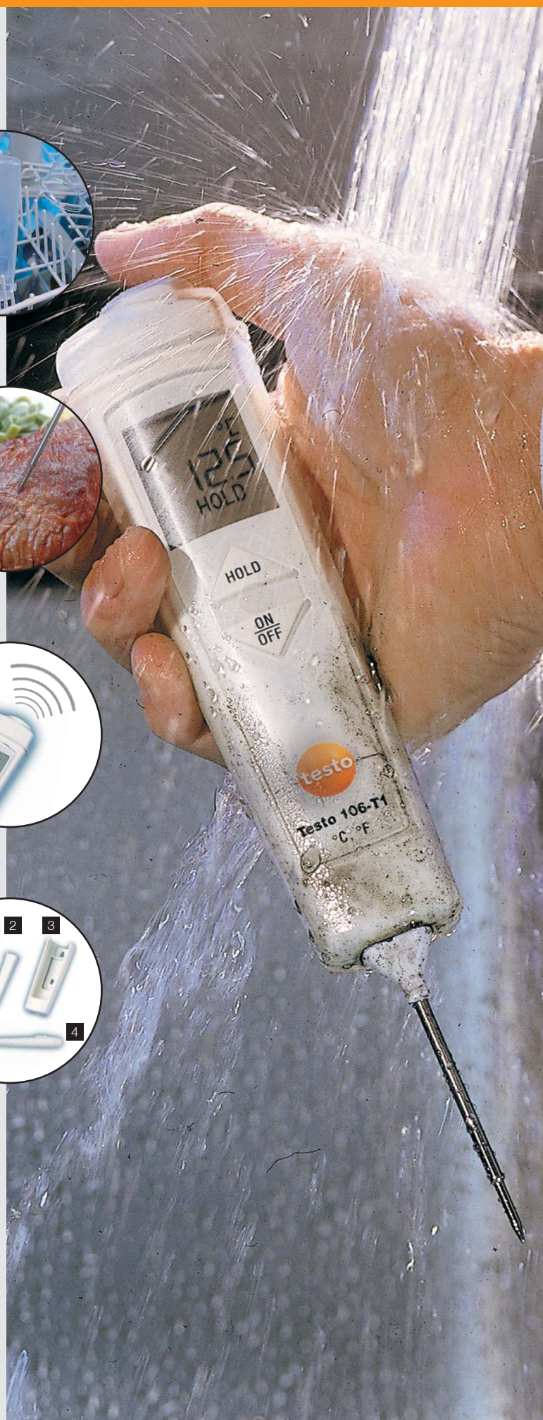
testo 106-T2 with audible alarm when limits are exceeded
