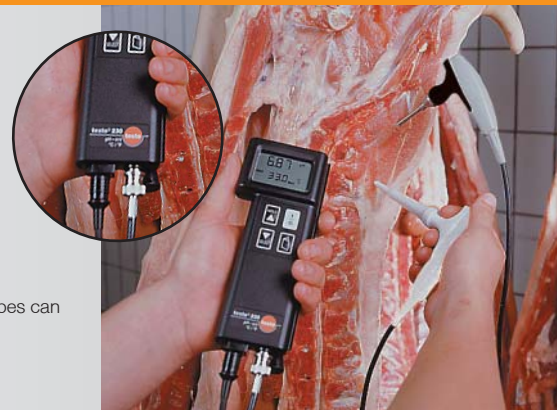
pH value and penetration temperature test on meat
