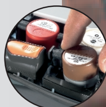
TÜV approved easy-to-change measurement cells
