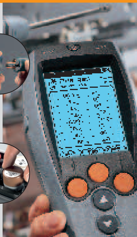
Fast checking of flue gas values in heating units
