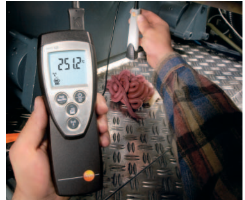
Temperature measurement in ductile materials with the superfast penetration probe, ideal for plastics, foodstuffs etc.
