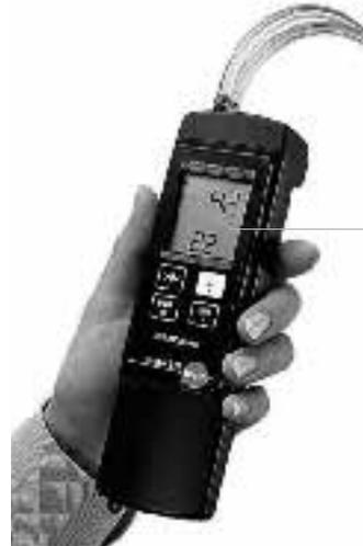
Simultaneous display of velocity and pressure value
